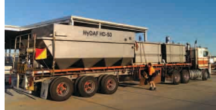
A Hydroflux Hy-DAF HD Dissolved Air Flotation (DAF) System being off loaded at a dairy in Victoria.
